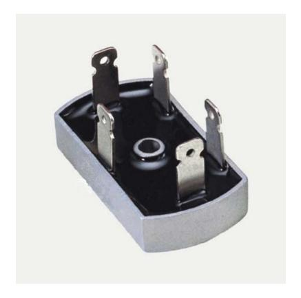
**NGAC G907-52** is an epoxy formulation designed for electrical encapsulating and potting applications. This low viscosity adhesive provides excellent flowability, surface wetting and minimal shrinkage upon cure
